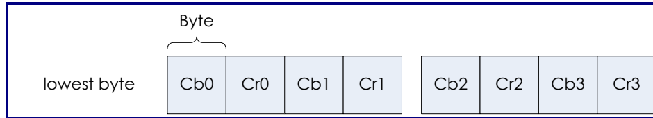
Figure 11-10. Semi-Planar Format of De-interleaved Chrominance
