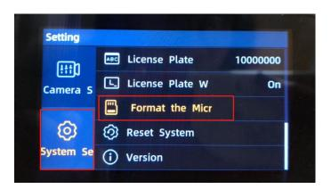
⑤ Press 0 to enter the menu. Press 0 to reach "OK" and then press 0 to finish formatting on the camera.
