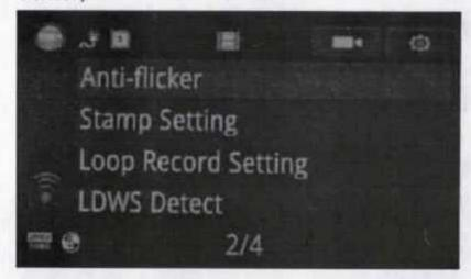
Frequency: Three modes: Auto/60Hz/50 Hz, the default is 50 Hz
