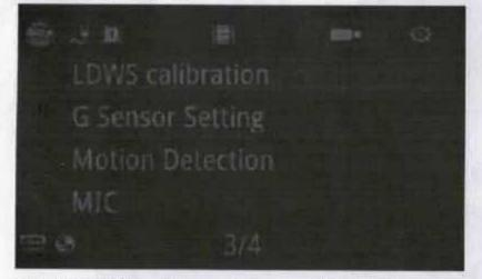
LDWS Calibration: show purple/red two lines, press up/down button directly to adjust the purple line, press MODE button then press up/down button to adjust the red lines. (only suitable for chipset A7LA50/A7LA70)
