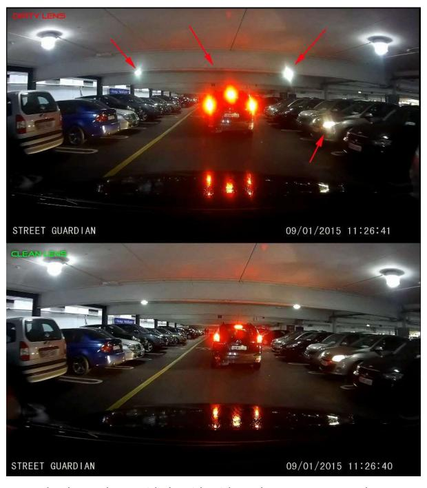
Example above shows side by side video where one camera has a single fingerprint on the lens, keeping the lens clean is imperative.
