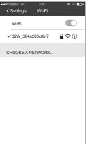
3. When the camera is connected with your smartphone, the Wi-Fi icon will turn green, and display your smartphone MAC address on the camera screen.
