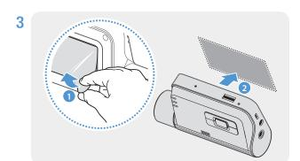
Remove the protective film from the adhesive mount, and then press the mount to the installation location.
