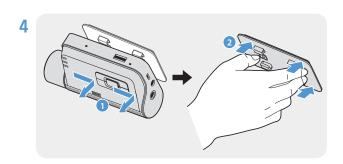
Remove the product from the mount and push the mount against the windshield to ensure that the mount is firmly fixed.
