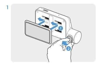
Align the mount to the mount rail on the product, and then slide it until you hear a click (1). Then, carefully remove the protective film (2).
