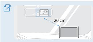
If a GPS navigating device is installed on the dashboard, its GPS reception may be affected depending on the dashboard camera's installation location.
