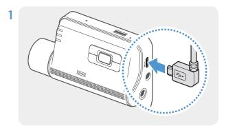
Connect one end of the rear camera cable to the front camera's V-IN port.
